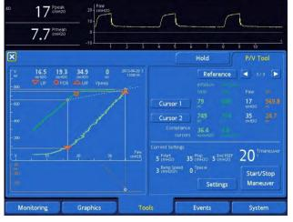
Graphic 1: A cursor function enables graphical analysis of the curve, including identification of inflection points
